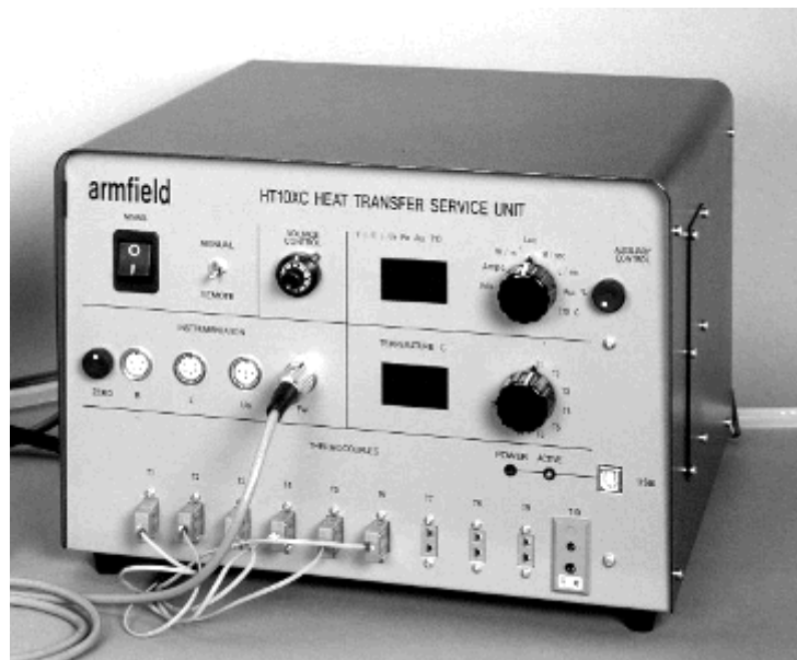
HT10XC Heat Transfer Service Unit (Connected to thermocouples T1 – T6 and to flow rate sensor Fw)
