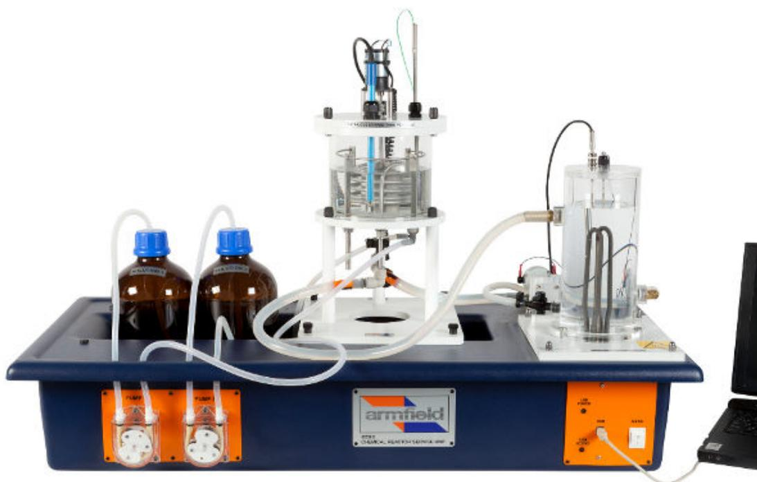
CEXC fitted with CEM MkII Continuous Stirred Tank Reactor
