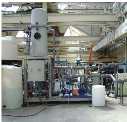
► New York City Dept. of Environmental Protection Ammonia Recovery Process test system at CASTion's Worcester, MA, facility. Since conducting the demonstration project in 1999 at Staten Island's Oakwood Beach wastewater treatment plant, the process has been improved using proprietary Controlled Air Separation Technology (CAST) followed by ion exchange.
