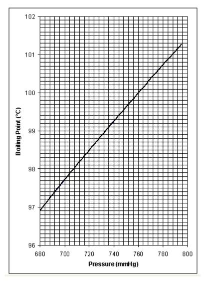
Boiling Point of Water (mm Hg-°C)
