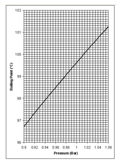
Boiling Point of Water (bar-°C)
