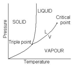
The saturation point of water is the condition at which a phase change occurs from liquid to vapour, or vapour to liquid. It occurs at a very precise set of conditions, which form a line when plotted on a graph such as that shown above (marked L V). Measurement of the saturation point therefore requires accurate measurement of absolute pressure and absolute temperature. Selection of suitable measuring devices must take into account several factors:
