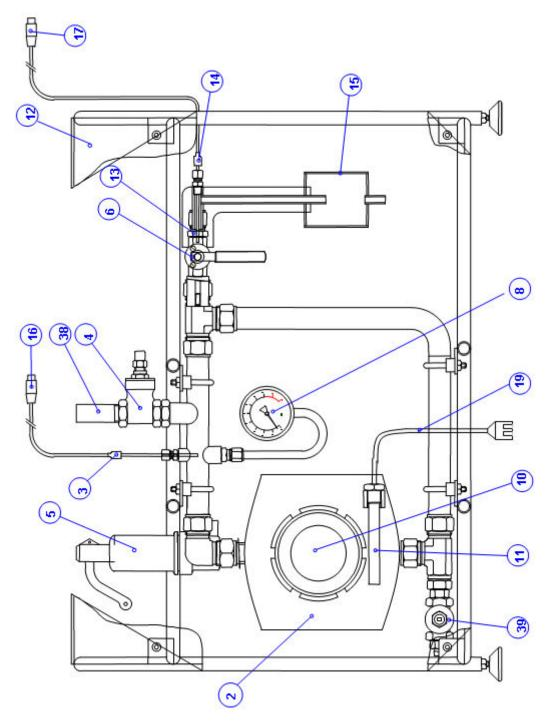
Figure 2: Side View of TH3 Saturation Pressure Apparatus
