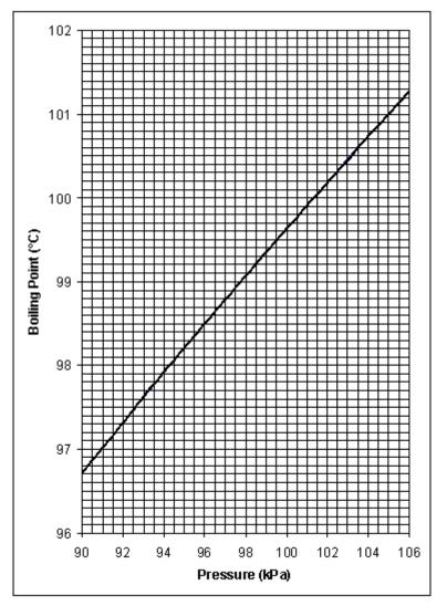
Boiling Point of Water (kPa-°C)
