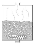
If the pressure is now reduced without a corresponding reduction in temperature, for example by bleeding off steam from the system, then the saturation temperature is reduced. The superheated liquid vaporises as the vapour point falls, producing violent frothing.
