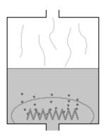
During this stage, small bubbles may occasionally be seen condensing on the sight glass.
