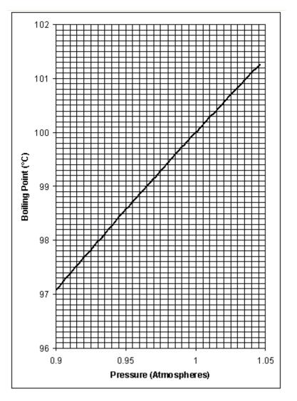
Boiling Point of Water (Atmospheres-°C)
