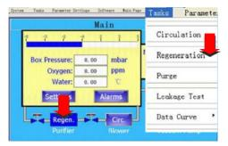
(2) Press Start Adjusting Gas Flow to adjust regeneration gas flow and press it again to finish the flow adjustment
