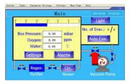
Two valves are interlocked. Turn on one valve will automatically turn of the other.
