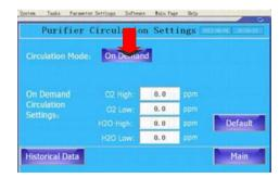
(3) Enter parameters and the purifier will work on demand to maintain the O2 and H2O within the set range
