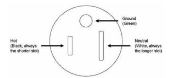
**FIGURE 7.1** Representative design for a three-wire grounded outlet. The design shown is for 15-A, 125-V service. The specific design will vary with amperage and voltage.
