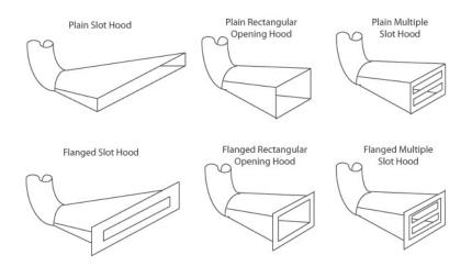
**FIGURE 9.12** Diagrams of typical slot hoods.
