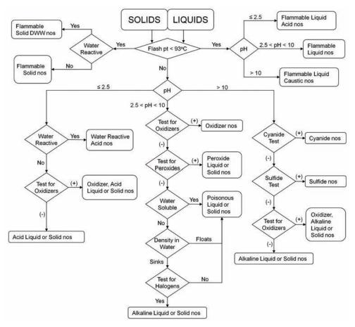
**FIGURE 8.1** Flowchart for categorizing unknown chemicals for waste disposal. This decision tree shows the sequence of tests to be performed to determine the appropriate hazard category of an unknown chemical. DWW, dangerous when wet; nos, not otherwise specified. Following categorization, select a hazard reduction procedure (section 8.D) or disposal option (section 8.B.6).
