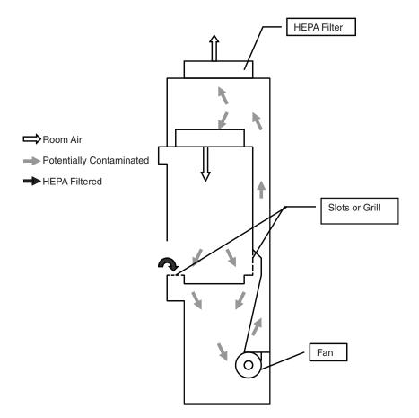
**FIGURE 9.13** Example of a Class II biosafety cabinet. Room air passes around the user through the grill at the front of the cabinet. Filtered air passes into the cabinet over the materials, providing a clean environment for the materials in the cabinet. Potentially contaminated air moves through the grill and slots, across the cabinet, and passes through HEPA filters.
