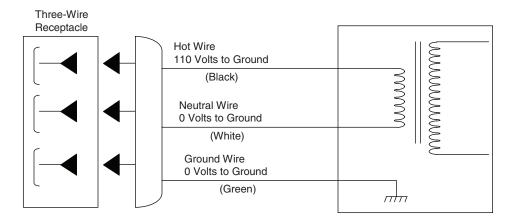
FIGURE 7.2 Standard wiring convention for 110-V electric power to equipment.
