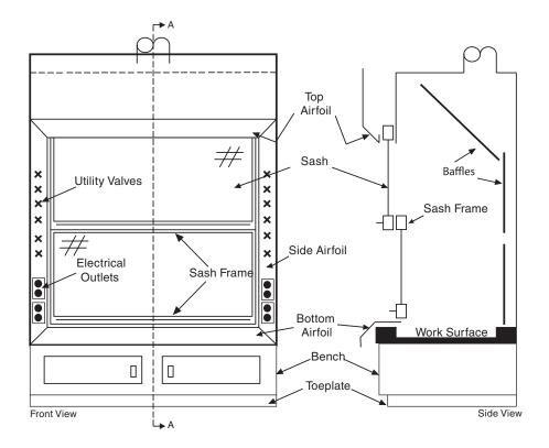
**FIGURE 9.8** Diagram of a typical distillation hood.
