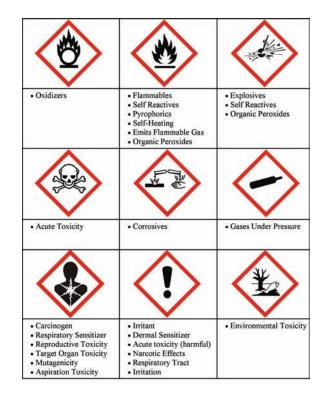
**FIGURE 4.1** GHS placards for labeling containers of hazardous chemicals.
