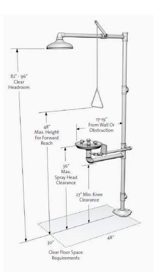
**FIGURE 9.2** Specifications for barrier-free safety showers and eyewash units.
