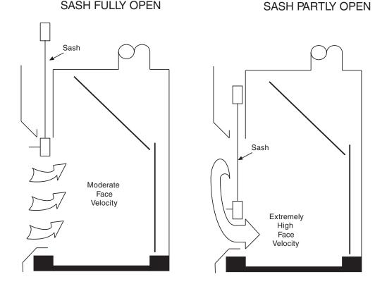
**FIGURE 9.5** Effect of sash placement on airflow in a nonbypass laboratory chemical hood.
