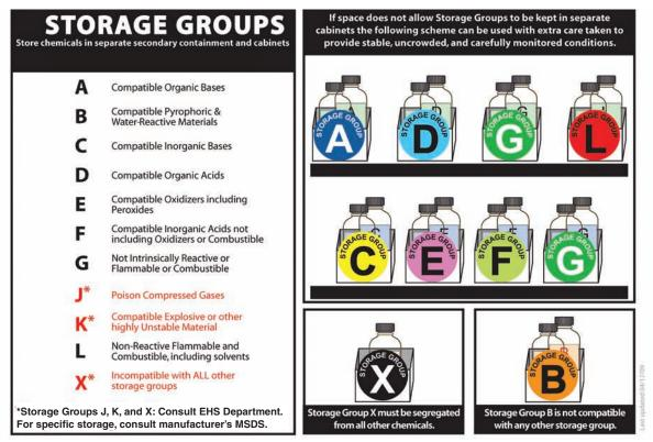
**FIGURE 5.1** Compatible storage group classification system. This system should be used in conjunction with specific storage conditions taken from the manufacturer's label and material safety data sheet. SOURCE: Adapted from Stanford University's ChemTracker Storage System. Used with permission from Lawrence M. Gibbs, Stanford University. NOTE: Also available on the CD accompanying this book.
