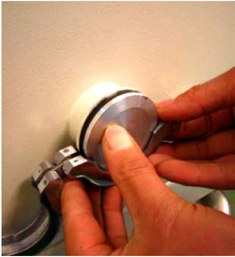
Remove the blanking flange on a feedthrough port of your choice.
