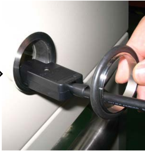
Feed the plug through the KF-40 O-ring and through the port.
