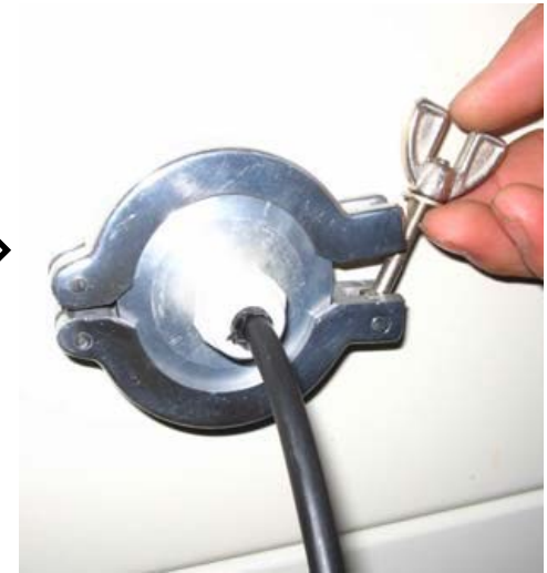
Slide the cable into the box until the flange on the cable mates with the KF-40 O-ring on the flange of the glovebox. Use a KF40 clamp to attach the two flanges firmly together.
