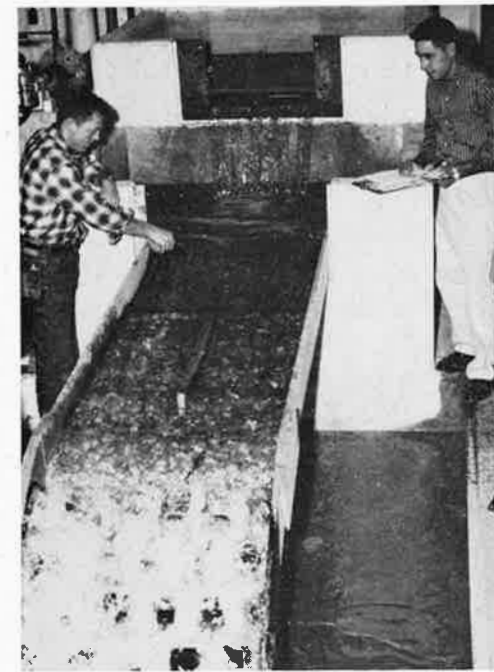
Huge volumes of water are delivered by this laboratory device to test models of structures used in hydraulics engineering.
