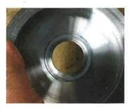
Also inspect and clean the back plate where the seal presses against it. Make sure any buildup of material is completey removed.
