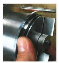
The back plate should push all the way against the rear housing while compressing the seal mechanism's spring. If the housing does not go all the way back, see step 6 and check the tab alignment.
