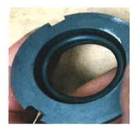
Inspect the "O" ring for any damage or build up. This "O" ring needs to sit firmly in the slot around the seal.
