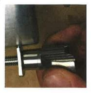
2. Remove the outside housing by pulling on the output neck
