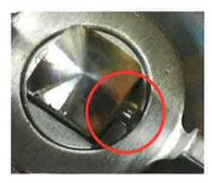
Allow the pin to slide to one side. This will hold the impeller and back plate in place.
