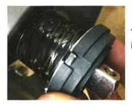
The seal mechanism is made up of four parts. The seal ring, the shaft O-ring located inside the seal, the seal holding cup, and the spring.
